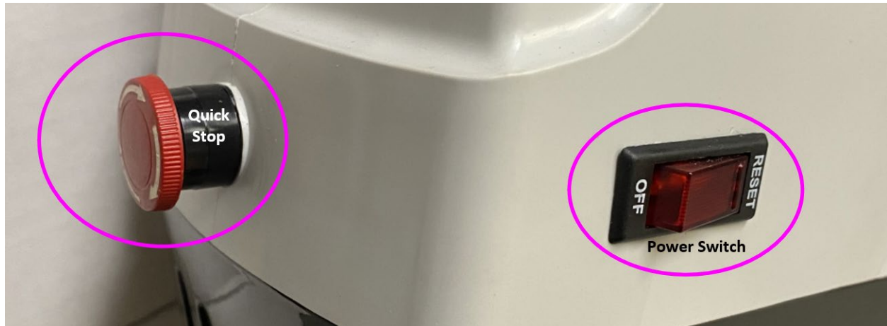
Figure 1: Location of Power Switch (in ON position) and Quick Stop Button
